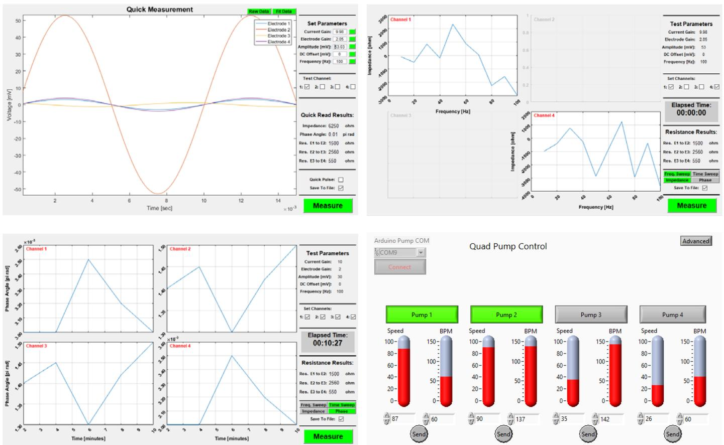
**Figure 3:** TEER parameter selection and calibration screen (upper left), frequency sweep screen with 2 of 4 channels selected (upper right), time sweep screen with all 4 channels selected (lower left) and interface for controlling fluid perfusion with up to four independent pump heads (lower right).
