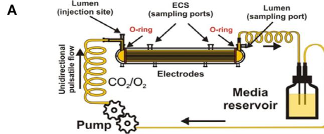
(A) Diagrammatic representation of the DIV-BBB. A bundle of porous polypropylene hollow fibers is suspended in the DIV-BBB chamber. The hollow fibers are in continuity with a medium source through a flow path consisting of gas-permeable silicon tubing. Two three-way stopcocks positioned on either side of the module regulate the access to the luminal compartment.
